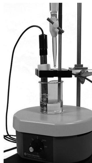
where the solution is mixing smoothly but gently. If the magnetic stirrer also has a heater function be certain that this remains off throughout this experiment.
