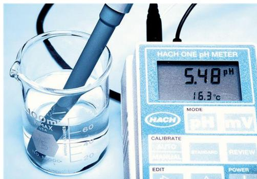
pH meters are used to measure pH values of water samples, such as determining acidity of rainwater samples. Rain water contains dissolved carbon dioxide that produces a weakly acidic solution. Rain naturally has a pH between 5 and 6. The pH of rain in parts of the U.S. is less than pH 5, which is harmful to aquatic life and human health. This is acid rain.
