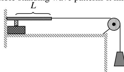
b) By measuring a segment of white string of known length, determine its density. Attach a piece of thread to the white cord that is two to three times its length. Using the density of the white cord and assuming a mass of 200g is hung over the pulley determine the allowed resonant frequencies of the system. Obtain numerical answers for the frequencies corresponding to the first four modes.
