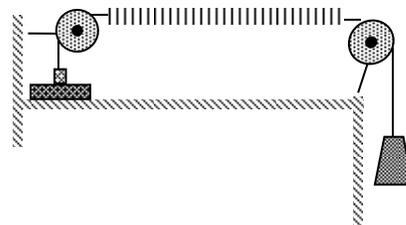
b) Locate the frequencies of two adjacent modes and use them to estimate the fundamental frequency of the system. Measure the mass  $M$  of the spring and its spring constant  $k$ .
