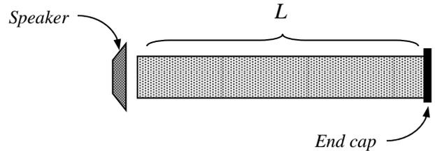
b) Measure the first three resonant frequencies of the tube. What speed of sound does each of these frequencies imply?
